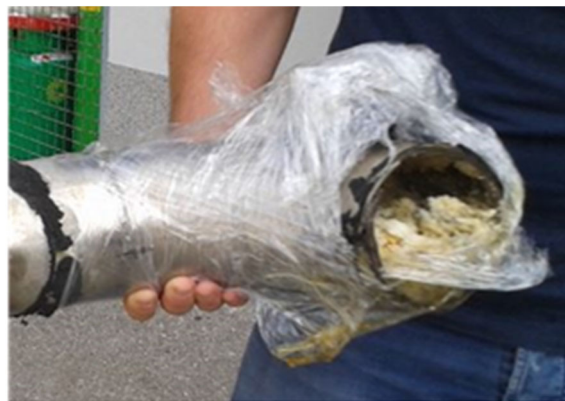
Ammonia carbamate formed in a pipe
